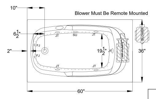
REMOTE MOUNTING THE BLOWER: If an extension cord is required, use a minimum 16 AWG cord with a maximum of 20ft length
