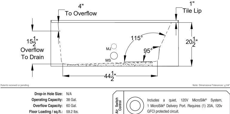
**Operating Capacity:** 38 Gal. Overflow Capacity: 60 Gal. Floor Loading / sq.ft.: 59.2 lbs. Carton Wt.: 125 lbs. Cube: 26.4 ft.<sup>3</sup>
