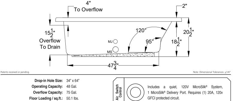
Overflow Capacity: 75 Gal. Floor Loading / sq.ft.: 50.1 lbs. Carton Wt.: 112 lbs. Cube: 34.3 ft.<sup>3</sup>
