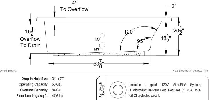
Construction: Reinforced Acrylic shell mounted on Level Form<sup>™</sup> pre-leveled full support base.
