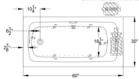
REMOTE MOUNTING THE BLOWER: If an extension cord is required use a minimum 16 AWG cord with a maximum of 20ft length
