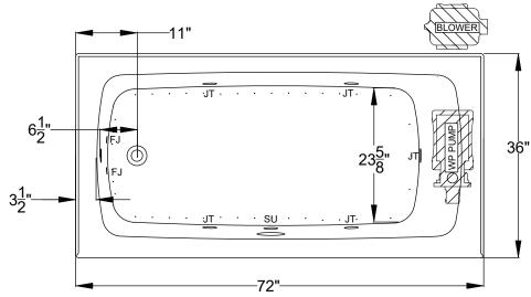
REMOTE MOUNTING THE BLOWER: If an extension cord is required, use a minimum 16 AWG cord with a maximum of 20ft length
