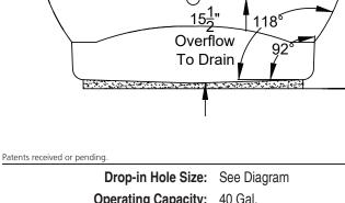
Operating Capacity: 40 Gal. Overflow Capacity: 61 Gal. Floor Loading / sq.ft.: 52.4 lbs. Carton Wt.: 146 lbs. Cube: 34.3 ft.<sup>3</sup>
