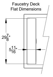
of the bath. Consult factory for details. Radius 3" 2" To Overflow Headrest 22" 18" Overflow 20" 105° To Drain
