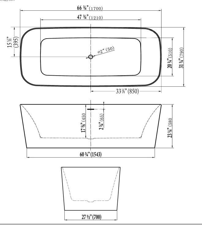
Overflow Capacity: 79 Gal. Floor Loading: 52.6 lb/ft²
