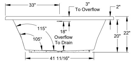
Includes Linear Overflow Drain Assembly
