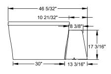
The Acrylic Equipment Cabinet is standard and required on MicroSilk® baths. Standard left-hand Acrylic Equipment Cabinet location shown. Please specify if optional right-hand location is desired.
