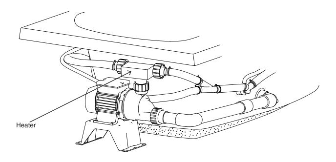
Jason's JT1000 1000 watt bath heater for Integrity™ Whirlpools automatically maintains water temperature while the whirlpool is in operation.
