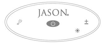
One main control touchpad mounted on the bath features several icons used by the bather to control the bath. This sheet will outline the functions of the system when a particular icon is pressed. If the icon is lit WHITE, then that particular option is available to operate. If the icon is lit BLUE, that particular option is currently in operation.
